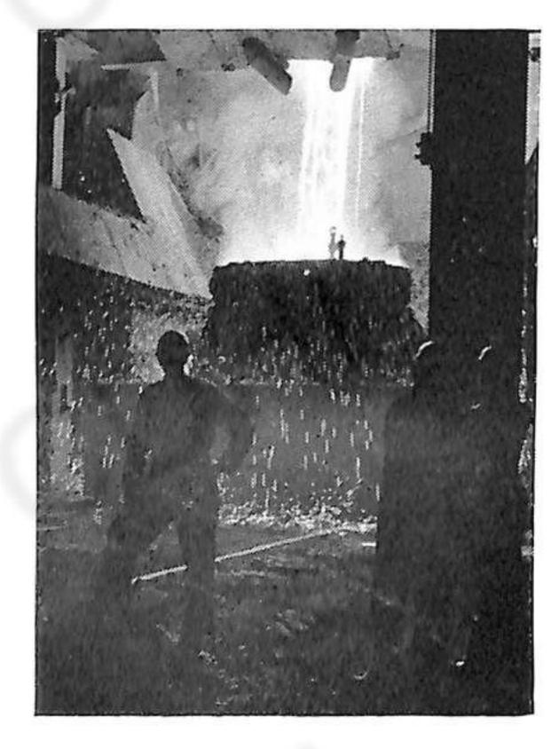
Above: Tapping a heat of steel from one of the Kaldo converters
